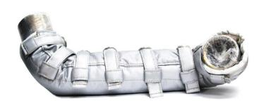
**DESCRIPTION:** Constructed of durable materials, this wrap is designed to handle up to 1000 °F of continuous heat while its exterior is excellent for fuel spills and UV performance. **ThermalMat-1000T** is an excellent solution for maintaining proper gas temperatures and touch protection. Stainless Steel mesh can be added if vibration or mechanical abrasion is a concern.
